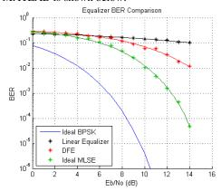
Run the linear equalizer, and plot the equalized signal spectrum, the BER, and the burst error performance for each data block. Note that as the Eb/No increases, the linearly equalized signal spectrum has a progressively deeper null. This highlights the fact that a linear equalizer must have many more taps to adequately equalize a channel with a deep null.
